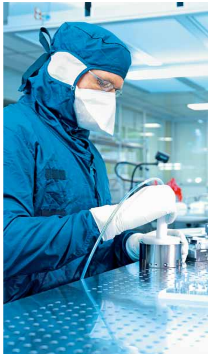
Assembly work performed in a class ISO 5 clean room
