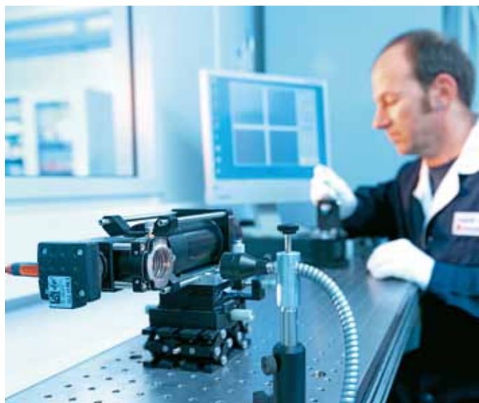
Assembly: Electronic adjustment of a reticle
